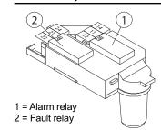
The relay module can be fitted into the module interface on the Gira smoke alarm device Dual detector and is powered via the connecting wires provided in the smoke detector. Each module interface can accommodate exactly one module, meaning that radio modules cannot be operated in smoke detectors at the same time as relay modules.
